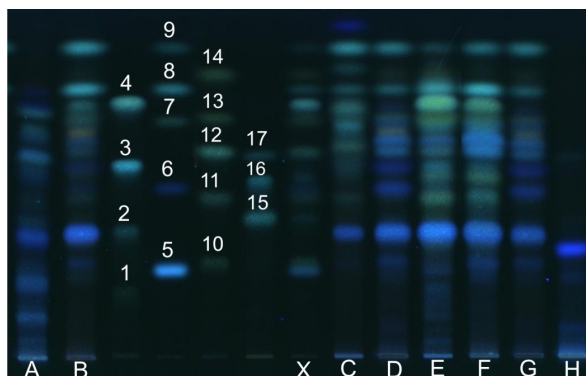
Fig. 1. Video-densitogram of TLC separation (silica gel 60 F 254 , hexane/ethyl acetate/formic acid (60:40:1.3, V/V/V), 2 % AlCl 3 , UV \lambda = 366 nm) of flavonoid standards and methanolic extracts of poplar buds: A – P. tremula , B – P. × canadensis 'Robusta', C – P. balsamifera , D – P. nigra 'Italica', E – P. × canadensis 'Marilandica', F – P. simonii , G – P. candicans , H – P. alba , X – the mixture of 17 standards. Key to the spots: 1 – myricetin, 2 – quercetin, 3 – kaempferol, 4 – galangin, 5 – chrysin 5,7-dimethylether, 6 – pinocembrin 5,7-dimethylether, 7 – pinobanksin, 8 – pinocembrin, 9 – pinostrobin, 10 – luteolin, 11 – apigenin, 12 – genkwanin, 13 – chrysin, 14 – tectochrysin, 15 – eriodictyol, 16 – isorhamnetin, 17 – naringenin.
