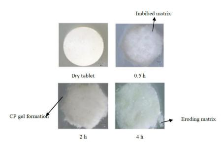
Fig. 6. Diagrammatic illustration of matrix and gel formation, breaking of small gel particles and matrix erosion during swelling of F10 at different time intervals when placed in 20 mL phosphate buffer solution, pH = 6.8 (taken with a Stereo zoom microscope).
