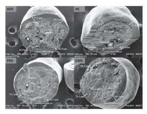
Fig. 4. SEM images of cut pellets. Standard numbers identify the coating thickness, underlined numbers identify the total pellet length.
