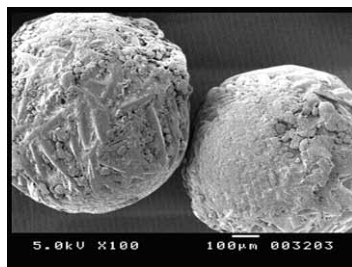
Fig 2. SEM image of fenofibrate lipospheres.
