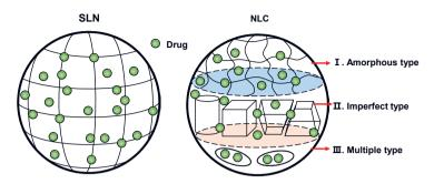
Fig. 1. Schematic of the internal structures of SLN and NLC. NLC – nanostructured lipid carrier, SLN – solid lipid nanoparticle.
