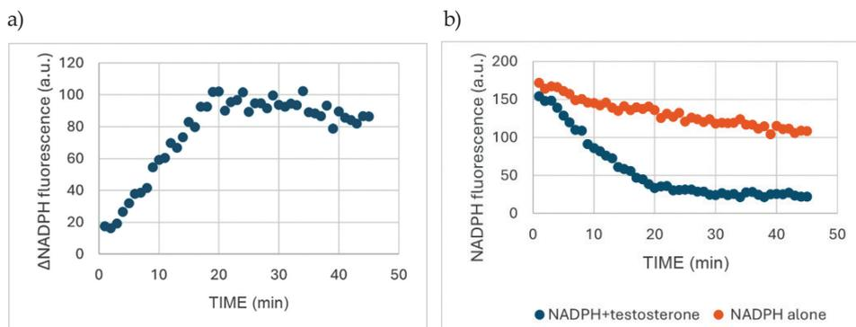
Fig. 5. Evaluation of AKR1D1 activity: a) change in NADPH fluorescence ( $\Delta$ NADPH) over time in the presence of testosterone, b) comparison of NADPH fluorescence over time in the presence of testosterone (blue) *vs.* its absence (orange).
