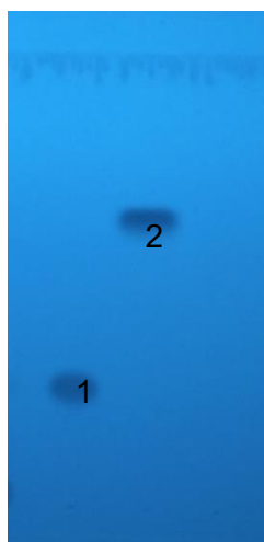
Fig. S3. RP-TLC chromatogram (mobile phase was prepared by mixing phosphate buffer saline (20 mM, pH 7.4) with methanol (30:70, V/V); detection – 254 nm; standard solutions – 100 \mu\text{g mL}^{-1} ; volume applied – 10 \mu\text{L} ). Legend: 1 – aloe-emodin, 2 – aloin A.
